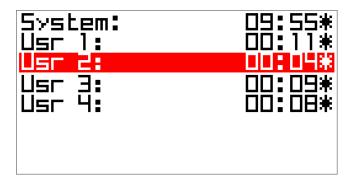
• To reset the odometer select it, scroll to "Clear" option and press "ENTER", the odometer resets as shown for "Usr 2" here below on the right.
