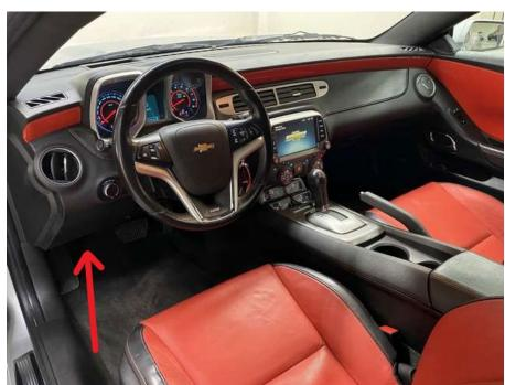
**OBDII pin connector**6
