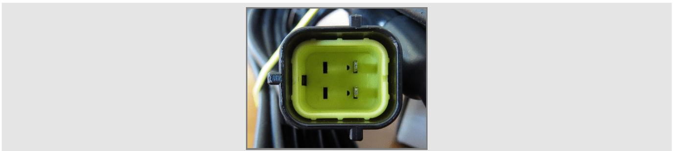
Mercury 849849 AXX interface cable has four not cabled wires you can connect to AiM devices.
