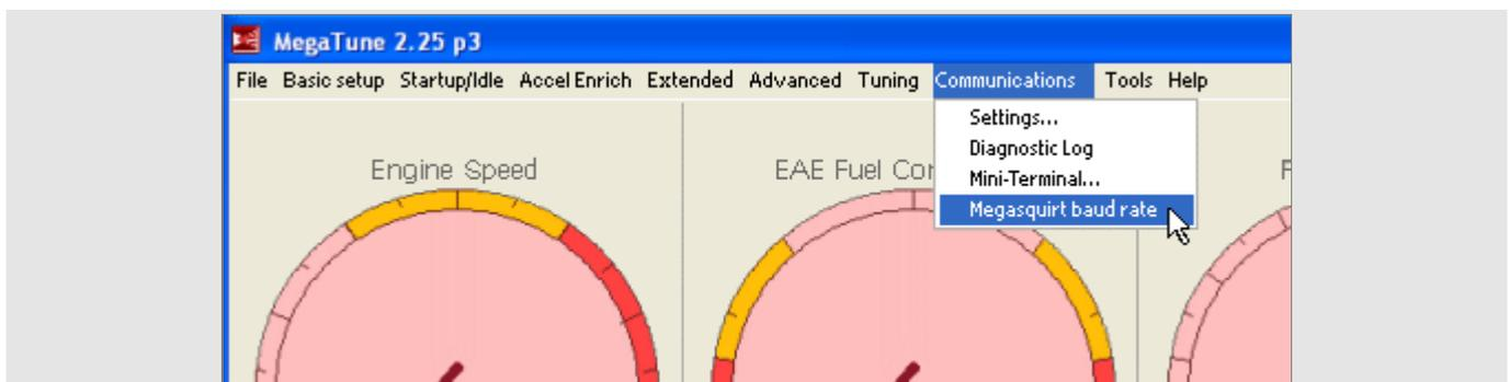
"Megasquirt baud rate" panel appears: set "baud rate -> 9600" and press "Burn to ECU" as shown here below.
