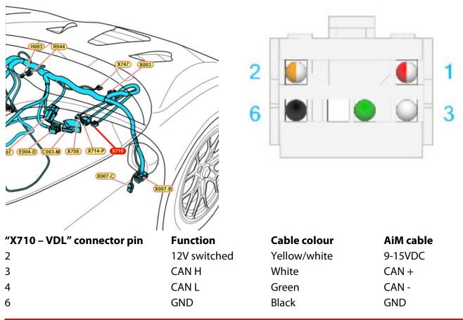
**N.B.:** to enable the CAN data output through the "X70 – VDL" connector, **the vehicle ECU firmware must be updated to the latest version available.**
