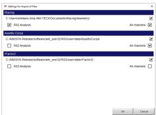
Flagging the RS2/RS3 checkboxes you will ask Race Studio to monitor the folder in which the simulator saves the telemetry files.
