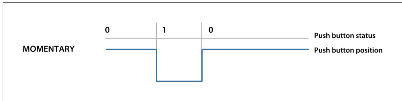
Setting the pushbutton as Momentary you can associate a Command to each pushbutton pressing the related button. Available command is "Device brightness" and the options are:
