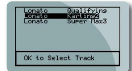
The desired track can be manually selected by pressing "OK".
