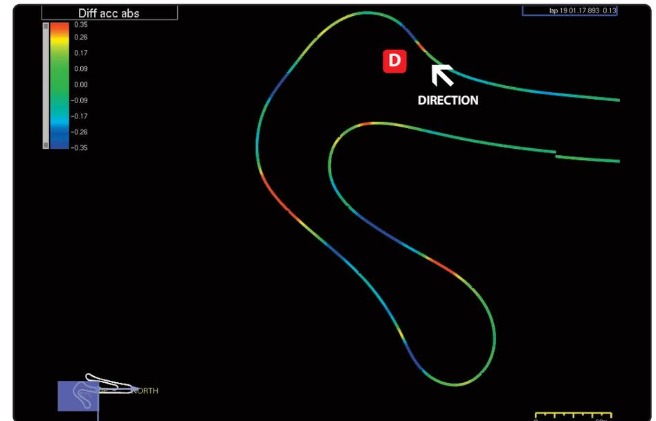
It's clearly evidenced how the vehicle reaches point **D** while braking after the straight line and understeer before entering the left corner in oversteering condition.
