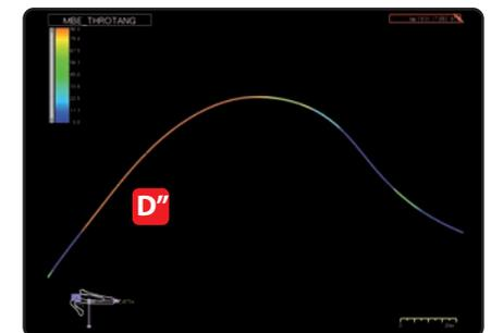
The strong oversteering behaviour at the entrance of the corner and the understeer while exiting, was caused by the wreck of front left shock absorber.
