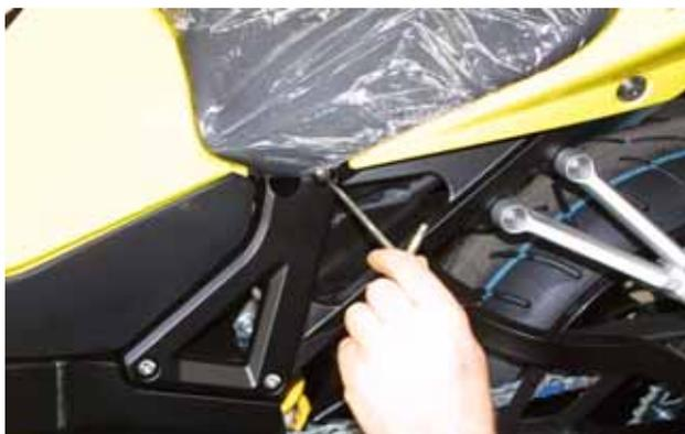
Figure 9: Unscrewing seats screw
