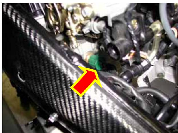
**Figure 19:** Water temperature connector – particular
