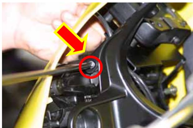
Figure 29: fixing the lateral screws
