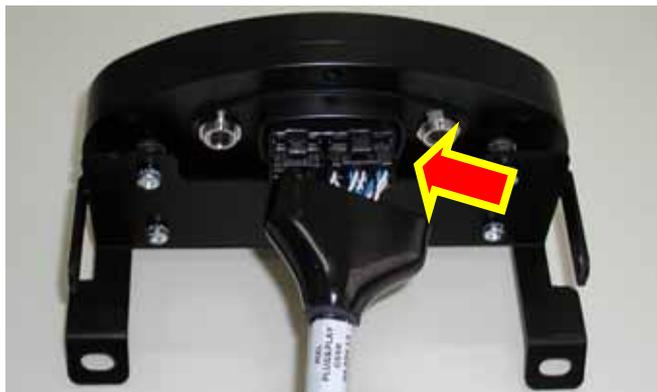
**Figure 23:** Wiring installation
