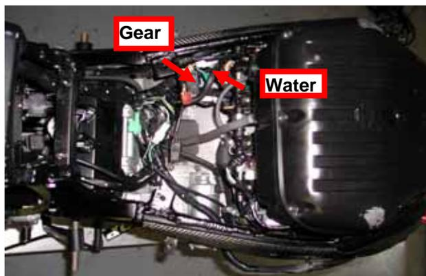
**Figure 17:** on board connectors – Water temp. / Gear
