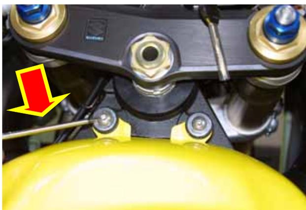
Figure 10: How to remove the gas tank
