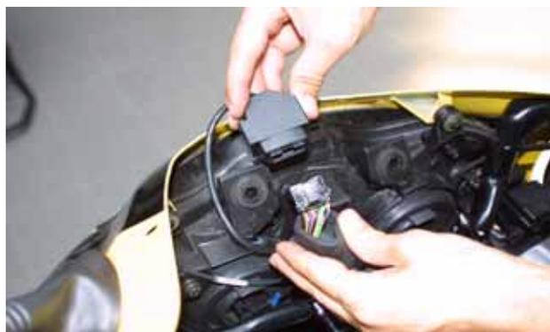
**Figure 26:** Wiring installation – particular of AMP connector
