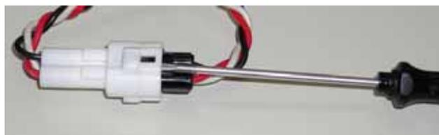
**Figure 20:** How to unplug a connector
