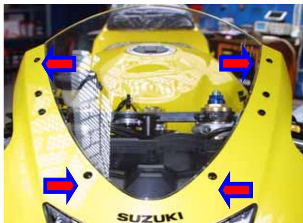
Figure 3: Front fairing – 4 Phillips recess screws.
