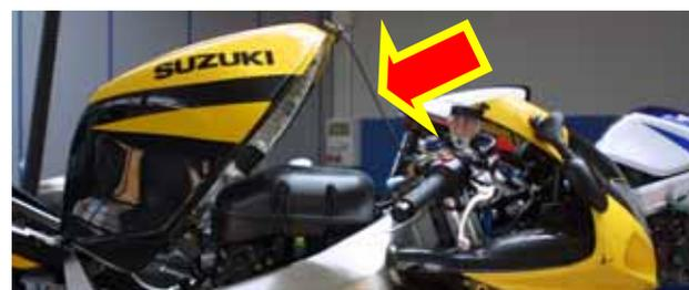
Figure 11: Uplifting the gas tank
