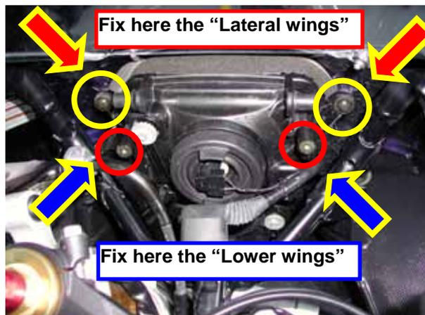
Figure 28: Lateral and lower “wings” fixing positions.
