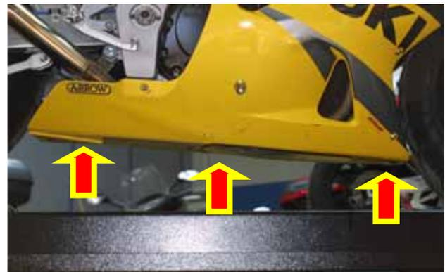
**Figure 5:** Junction between the fairings – pins location.
