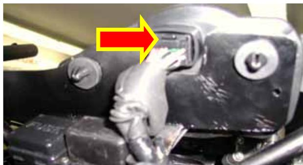
**Figure 16:** unplugging the on board dash connector
