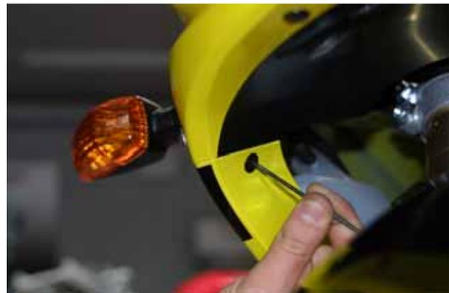
**Figure 6:** Unlocking the central clip of the plastic pin.
