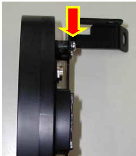
Figure 21: anti-vibration mountings – particular
