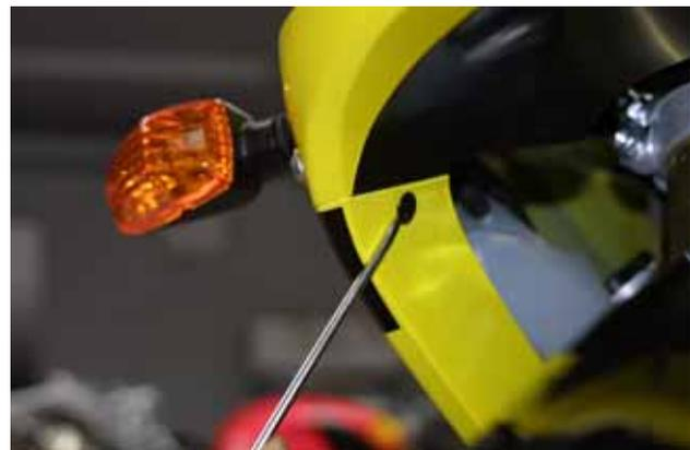
**Figure 7:** removing the plastic pin
