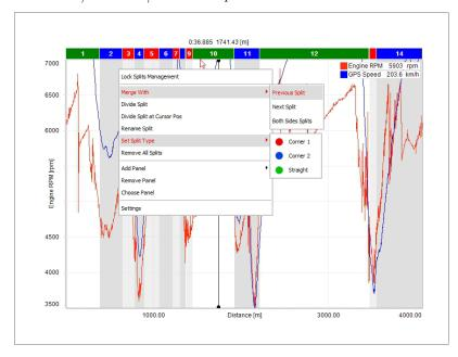
Double clicking on a split of the split bar the graph resizes at that split level and so does the track map bottom left of the software view; clicking again on the split bar the graph and the track map are resized back.
