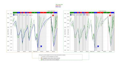
Min/Max values tags are three boxes that shows min/max and average value of the channel; the point where the min/max value has been sampled can be indicated; available options are:
