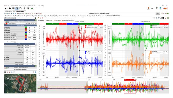
This layout comes by default with a Channels and Laps List Panel (1), a Track Map Panel (2), a Suspension Analisys Panel (3) and a StoryBoard Panel (4).
