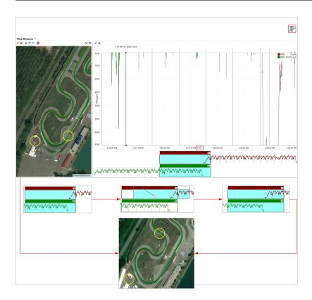
In "Local timing off" mode the X axis can show "Time" or "distance", the graph can be in snap on/off mode and the storyboard selects a fixed range of time; the graph can be zoomed in/out with the mouse wheel. dragging and dropping the selection in the storyboard the slice of race shown in the graph is moved as explained before.
