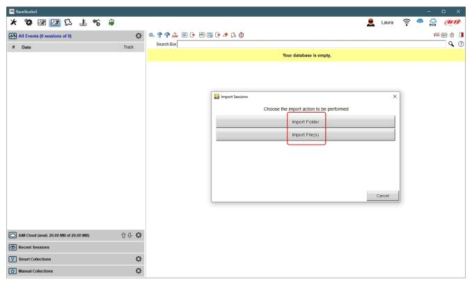
It is possible to import single files or entire folders of data. Pressing one of the buttons highlighted browse windows is prompted: select the file/folder to import and press OK. A window with a progress bar appears. In case the files are already in the database or if there is any issue the software warns you.
