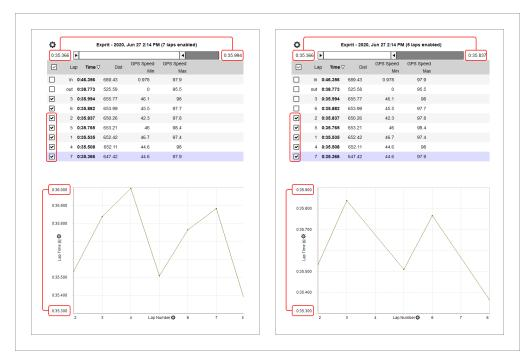
This views allows to add/remove a channel in the table top of the graph and to change the channel plotted on "Y" axis
