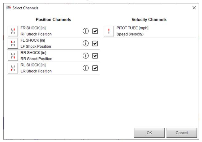
The suspension analysis panel puts together a time/distance plot of the suspension related channels (shock positions and/or velocities), a histogram of the same channels, the frequency analysis plot of the same channels and a logsheet with the main settings related to suspension analysis.
