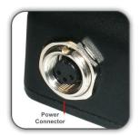
**SoloDL** features two connectors on the bottom of the system: one to connect to an external CAN expansion (for example SmartyCam – see Chapter 11) and the second is used for ECU connection and power (bottom right image). Please, take note that the external power can be received from the first or the second connector.
