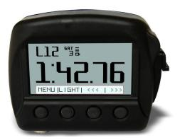
The menu activation is triggered whenever any of the four buttons is engaged; after four seconds, the menu will recede.
